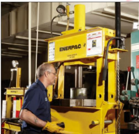
◀ An Enerpac H-Frame press quickly removes the shaft from this assembly.
