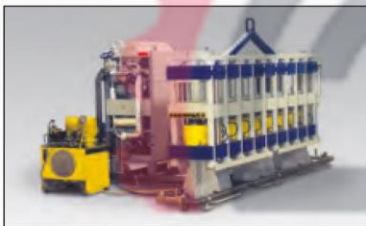
◀ Fully Automated PLC-Controlled 1800-Ton, High-Accuracy Press
