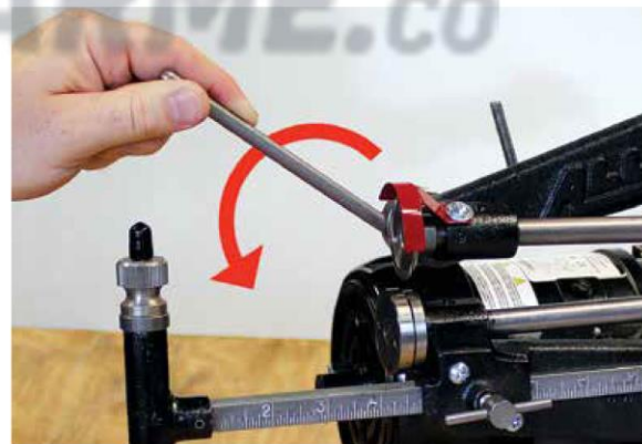
(Figure 4) Disengage the top cutting disc by rotating the cutter disc lever counter-clockwise.
