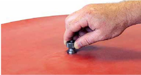
(Figure 5) Unscrew and remove the scale bar knurled nut from the scale bar assembly. Using the guide hole, position the gasket material onto the threaded scale bar spindle. Screw the knurled nut back onto the spindle to firmly secure the material. Hand tighten.
