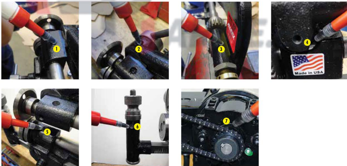
(Figure 16) The Motorized M3 is pre-lubricated at the factory. Like any piece of precision machinery, regular cleaning and lubrication of all gears, and moving parts is recommended. Light machine oil should periodically be applied to points 1, 2, 3, 4, 5, 6 and 7. Replace worn parts as necessary.
