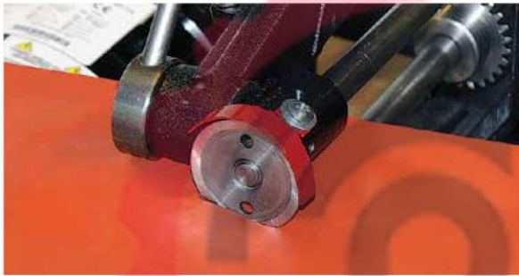
(Figure 6) To cut the OD, engage the top cutting disc by rotating the cutting disc lever clockwise. The top cutting disc should now penetrate the gasket material and is now in the proper position for cutting.
