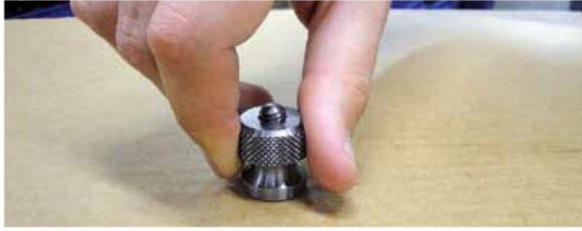
(Figure 4) Unscrew and remove the scale bar knurled nut from the scale bar assembly.
