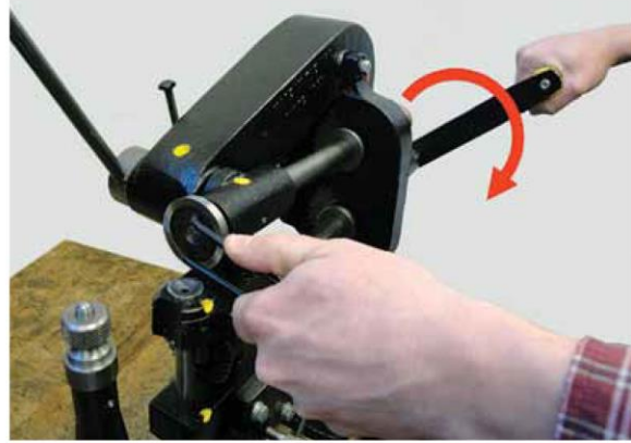
(Figure 11) Disengage cutting disc lever. Use spanner wrench (included) and place into corresponding holes in top cutting disc. The top cutting disc is loosened by holding spanner wrench and turning the crank handle counter-clockwise. It may be necessary to give the crank handle a sharp blow with the palm of your hand to initially loosen the cutting disc. Place new or sharpened cutting disc onto top shaft and tighten by holding with spanner wrench and turning crank handle clockwise.
