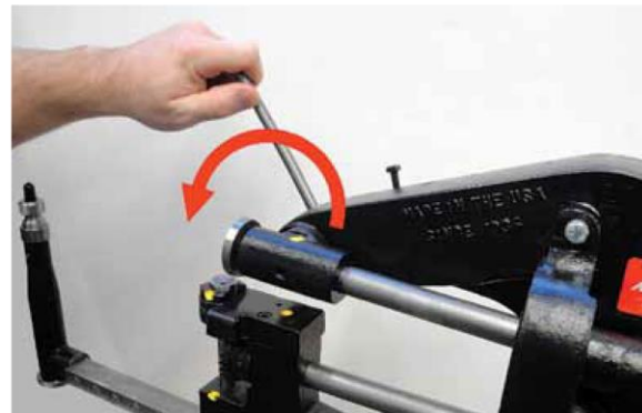
(Figure 4) Disengage the top cutting disc by rotating the cutting disc lever counter-clockwise.
