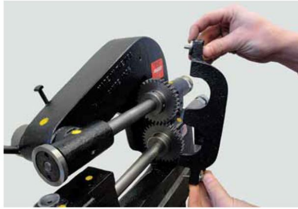
(Figure 10B) Remove gear guard by loosening two hex head cap screws using 7/16" wrench. Pull off gear guard.
