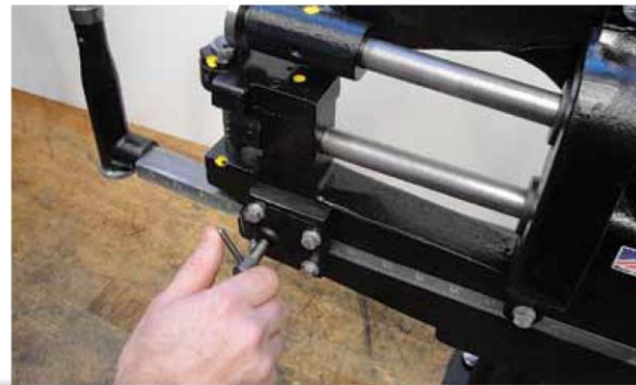
(Figure 3) Loosen the scale bar T-screw and slide the scale bar to the desired OD setting. Hand tighten the T-screw.
