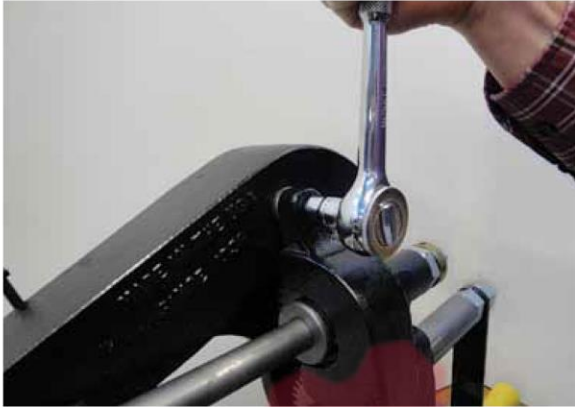
(Figure 10A) To replace the bottom cutter, other components of the unit must be removed first to gain access to the bottom cutter.
