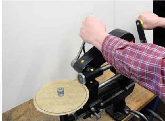
(Figure 8) To cut the inner diameter (ID), loosen the scale bar T-screw, and slide the scale bar to the desired setting. Hand tighten the scale bar T-screw. Engage the top cutting disc. Turn the hand crank, simultaneously maintaining downwards pressure on the cutting disc lever as before. Continue cranking until the entire ID of the gasket material has been cut. Disengage the top cutting disc and remove the newly cut gasket. Unscrew and remove knurled nut from spindle. Discard unwanted material.
