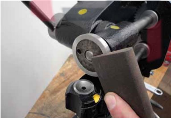
(Figure 12) Sharpen by holding a small, hand sharpening stone to bevel side of the cutting disc. Slowly turn the hand crank. Then hold the stone to the flat face to remove rolled edges or burrs.
