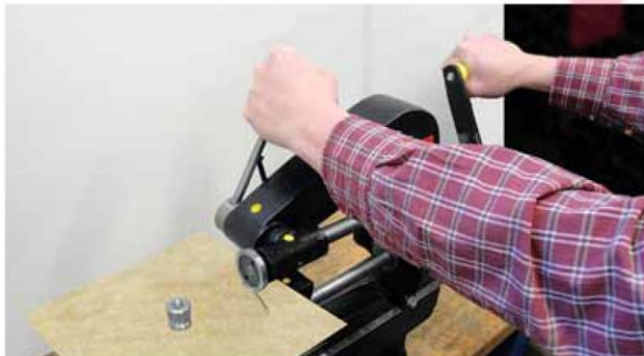
(Figure 7) Turn the hand crank clockwise. Simultaneously, with the other hand, maintain a constant downward pressure on the cutting disc lever. As the cutting discs rotate, the gasket material will be drawn towards the cutting discs initiating the cutting process. Continue cranking until the entire OD of the gasket material has been cut. Disengage the top cutting disc. Discard unwanted material.
