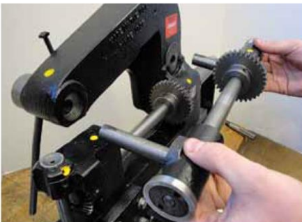
(Figure 10E) Slide top shaft assembly out of the frame assembly.
