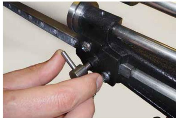
(Figure 3) Loosen the scale bar T-screw and slide the scale bar to the desired OD setting. Hand tighten the T-screw.
